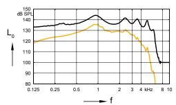
Max. Output sound pressure level  $(L_1 = 90 dB)$
