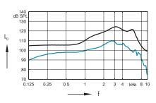
Output sound pressure level (L<sub>1</sub> = 90 dB)
