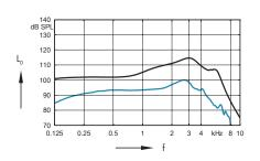
Output sound pressure level  $(L_1 = 90 \text{ dB})$
